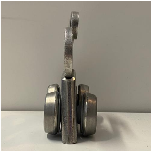
Shock absorber is twisted
