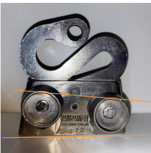
The wheels do not stay in their upper position with the help of spring force
