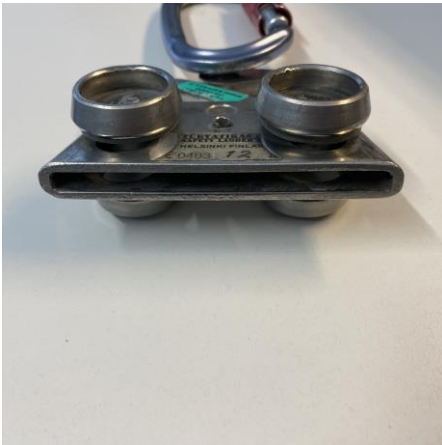
Support plate is missing
